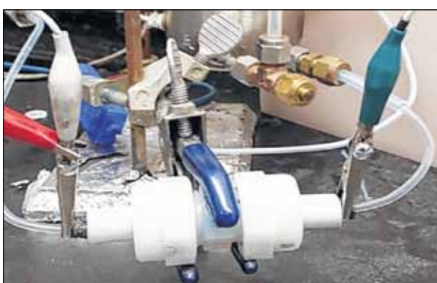
ABOVE, Stephen Creager's miniature fuel cell will be used with graphene to separate isotopes of hydrogen. BELOW, SRNL researchers work in lab with a Clemson grad student. The researchers' study is supported by the U.S. Department of Energy.
